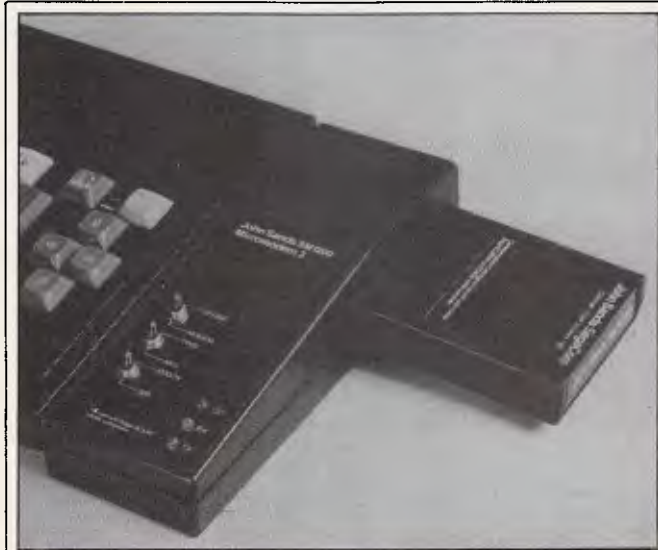
This is a thinly disguised Acme modem connected to John Sands' Sega home computer. Together, says John Sands, they become the John Sands Communications System. It can access videotex databases such as Viatel, Elders Farmlink, Microtex, and Aftel plus Teletel databases and bulletin boards.
